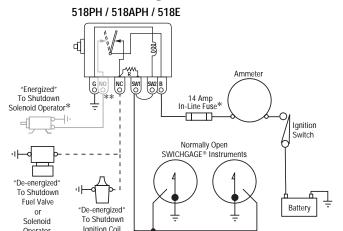
\* In-Line Fuse should be removed on "energized" to shutdown configurations
